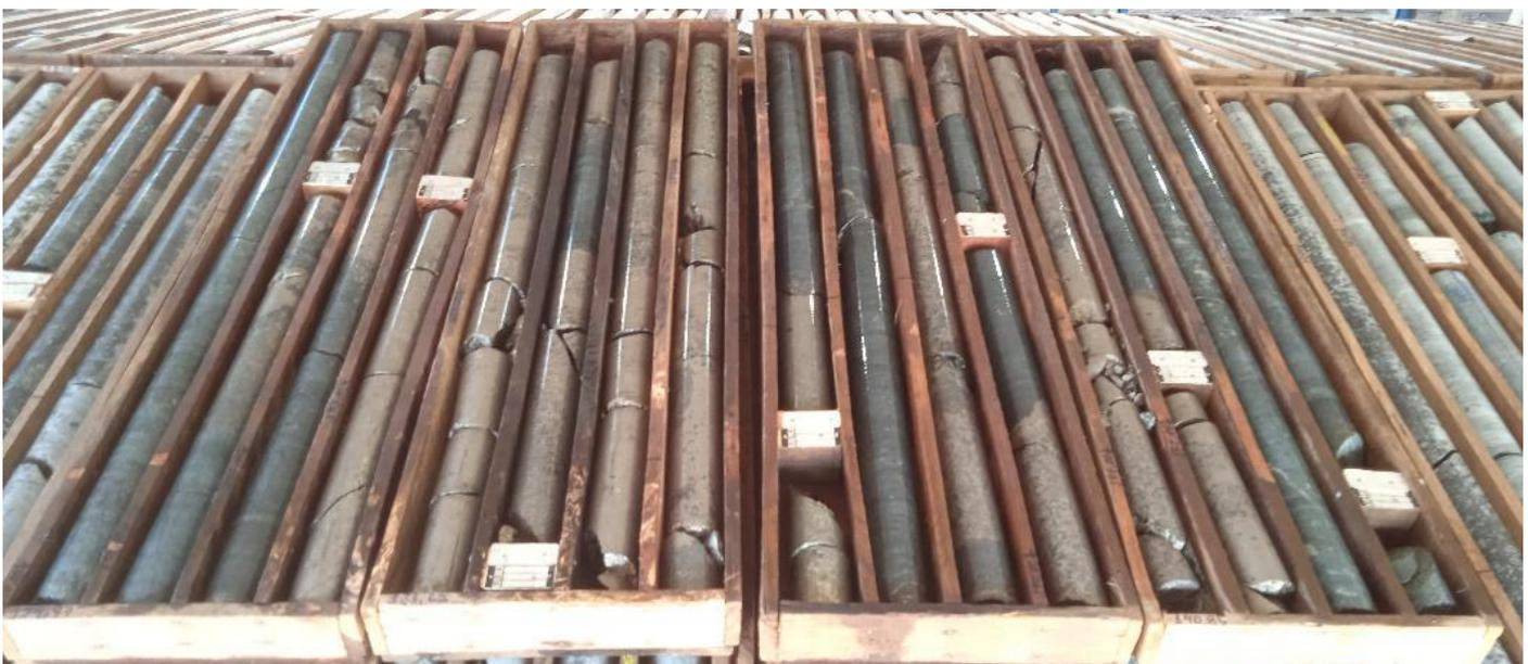
**DDH22LU047: Drill core showing massive and brecciated semi massive sulphides, from 131.1m to 142.1m\***
