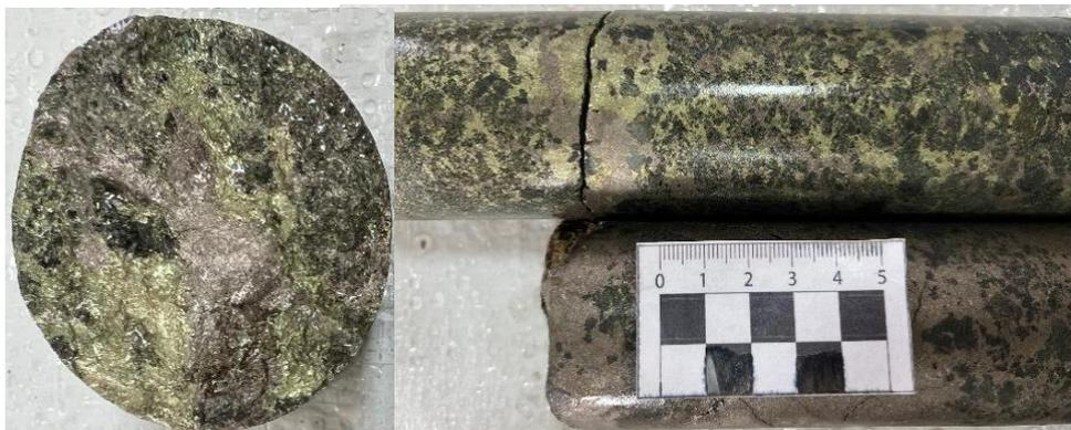
**DDH22LU047: High grade breccia semi-massive sulphide nickel-copper mineralization, from at 137.0m\***
