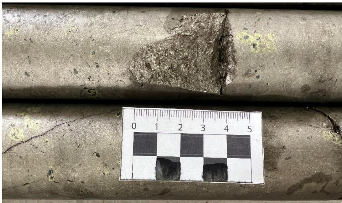
**DDH22LU047: High grade massive sulphide nickel mineralization at 136.0m\***
