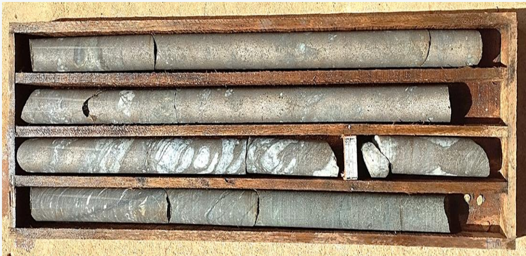
DDH2406T002 Massive/Semi-massive/ breccia sulphide mineralization at T6 target (57.0 – 60.7m shown).
