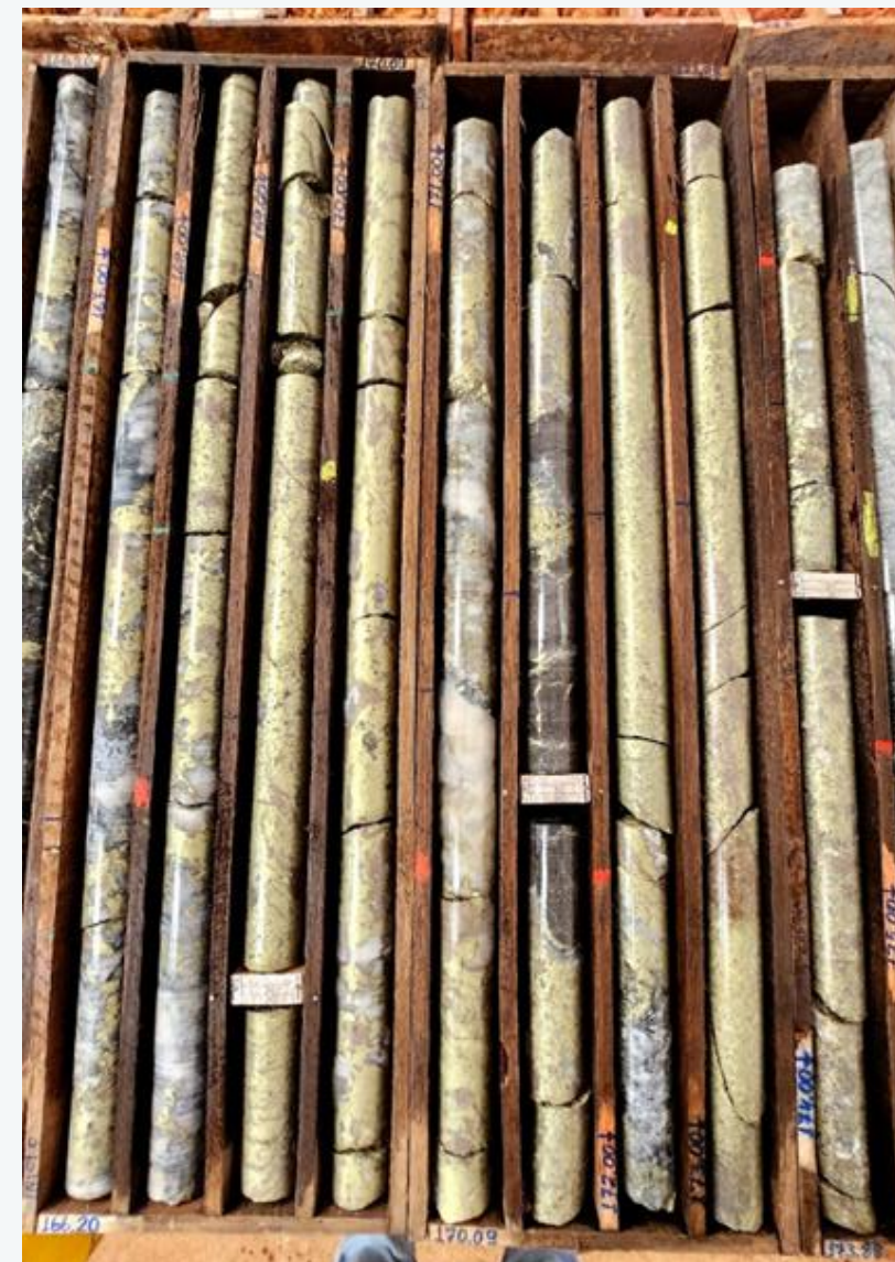
Massive/semi-massive/ breccia sulphide Cu mineralization at the T5 target (165.8 – 174.8m downhole shown).
