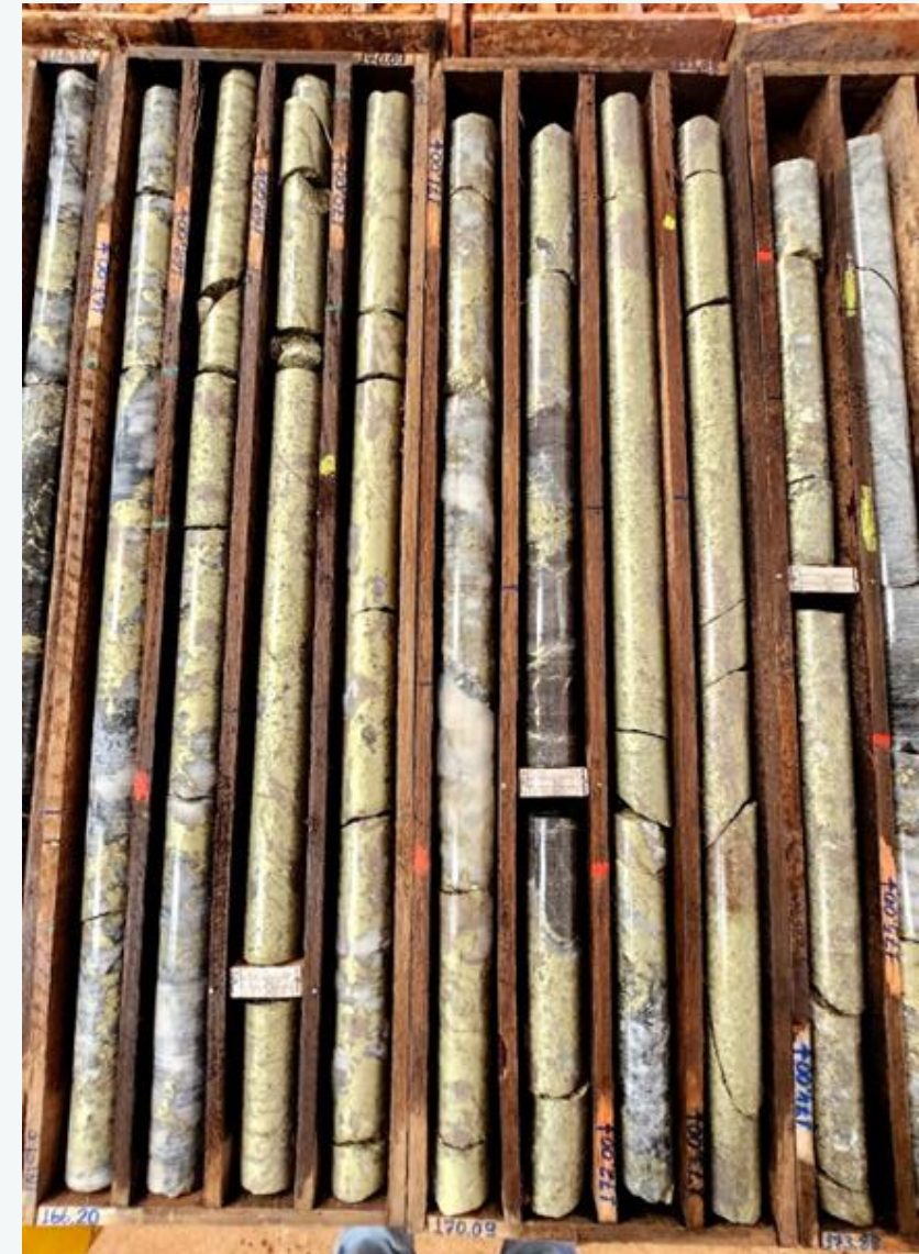
Massive/semi-massive/ breccia sulphide Cu mineralization at the T5 target (165.8 – 174.8m downhole shown).
