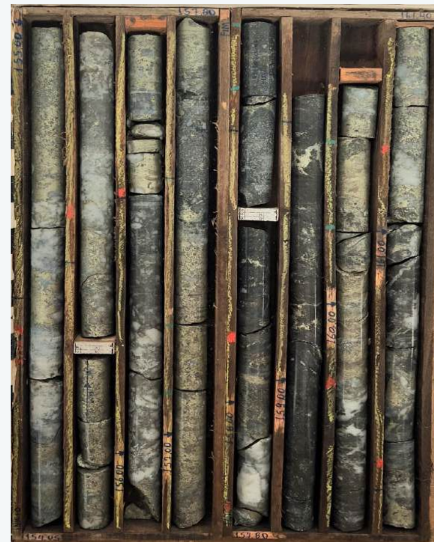
Massive/Semi-massive/ breccia sulphide Cu mineralization at T5 target (154.0 – 161.4m downhole).
