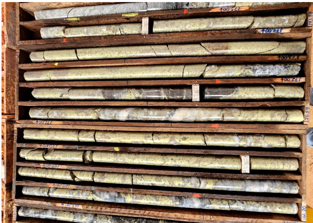
Figure 2: DDH2405T002 - Massive/semi-massive/ breccia sulphide Cu mineralization at the T5 target (165.8 – 174.8m downhole shown).
