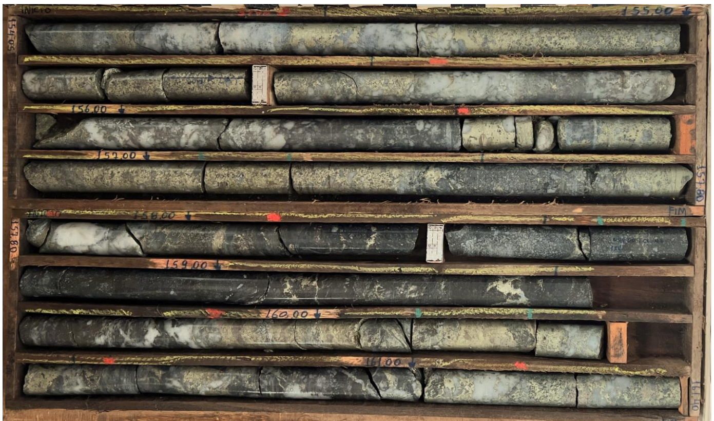
Figure 2: DDH2405T004 - Massive/Semi-massive/ breccia sulphide Cu mineralization at T5 target (154.0 – 161.4m shown).
