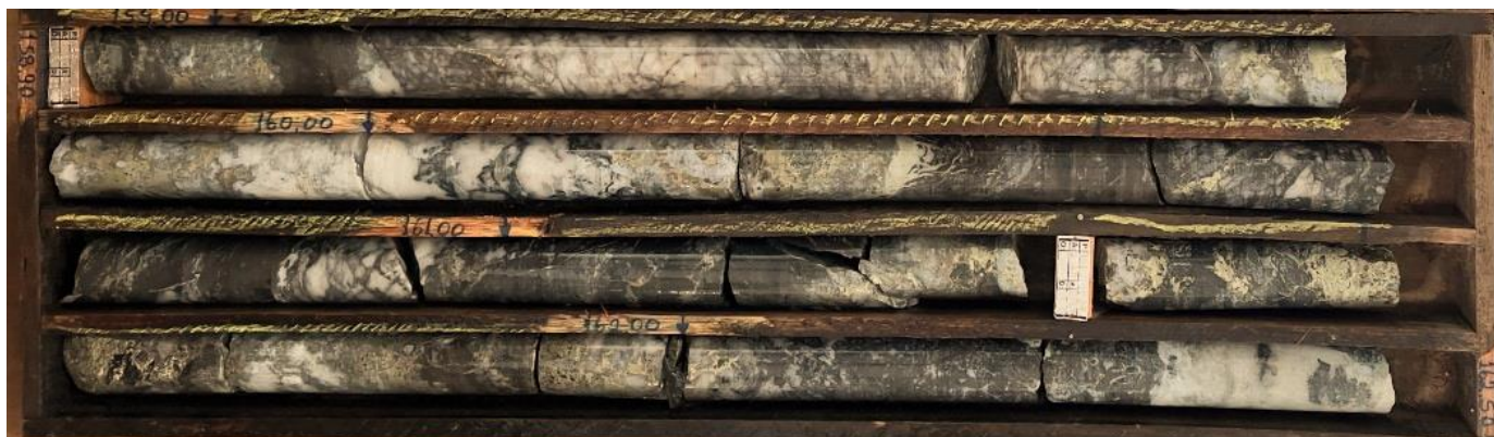
Figure 3: Breccia copper sulphides (results pending) in DH2405T003 (158.9 – 162.5m shown).
