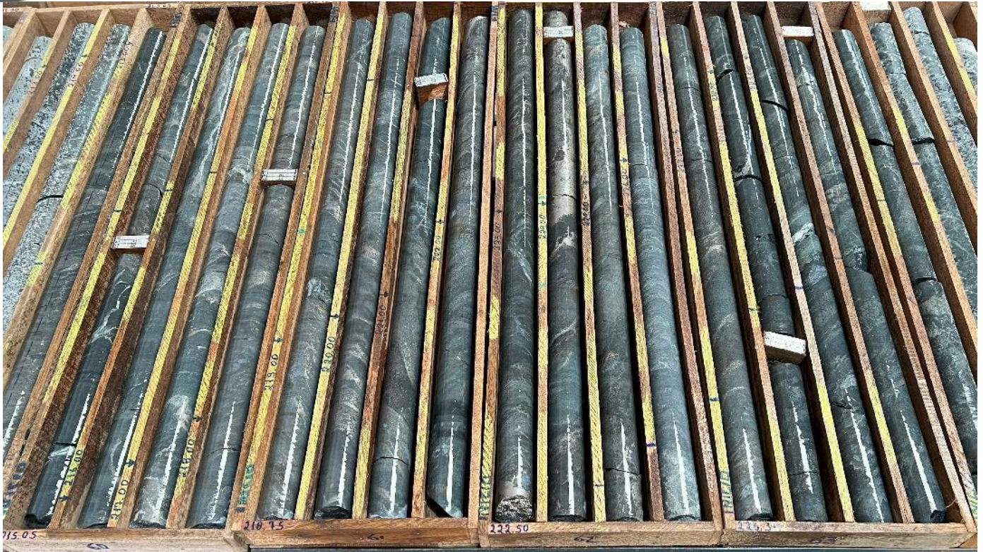
Figure 6: DDH2411T002 Sulphide mineralization – patches and veins, locally reaching massive/semi-massive (215m to 230m shown).
