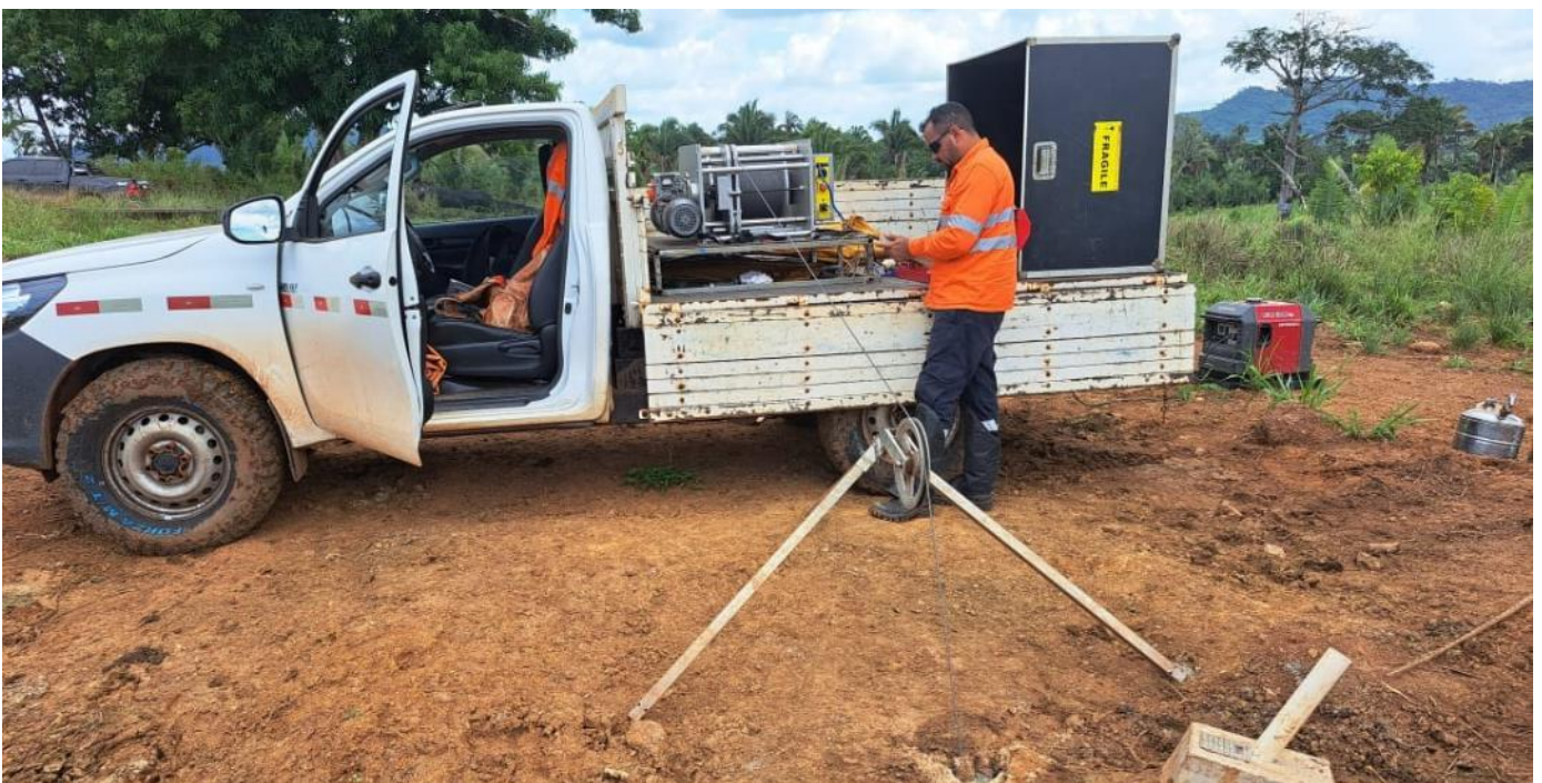
Figure 4: BHEM survey team in operation at the T5 Target – drill holes DDH2405T003, DDH2405T004, DDH2405T005 and DDH2405T006.
