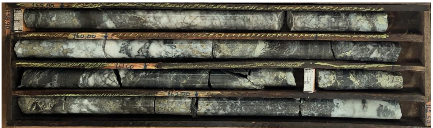
Figure 2: Breccia copper sulphides in DH2405T003 (158.9 – 162.5m shown).
