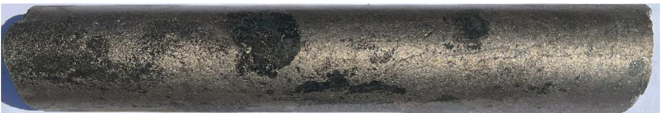
Figure 1: Massive sulphide mineralization in DDH2411T002 at T11 (224.1m to 224.4m downhole). Open along strike and at depth.
