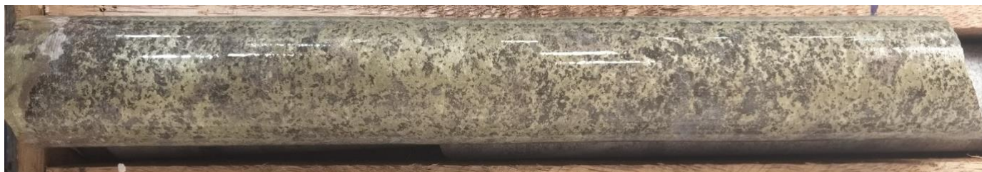
Figure 1: Interpreted breccia copper sulphide mineralization in DDH2405T012 at T5 (158.90m - 159.10m downhole), on the eastern most extent of drilling.
