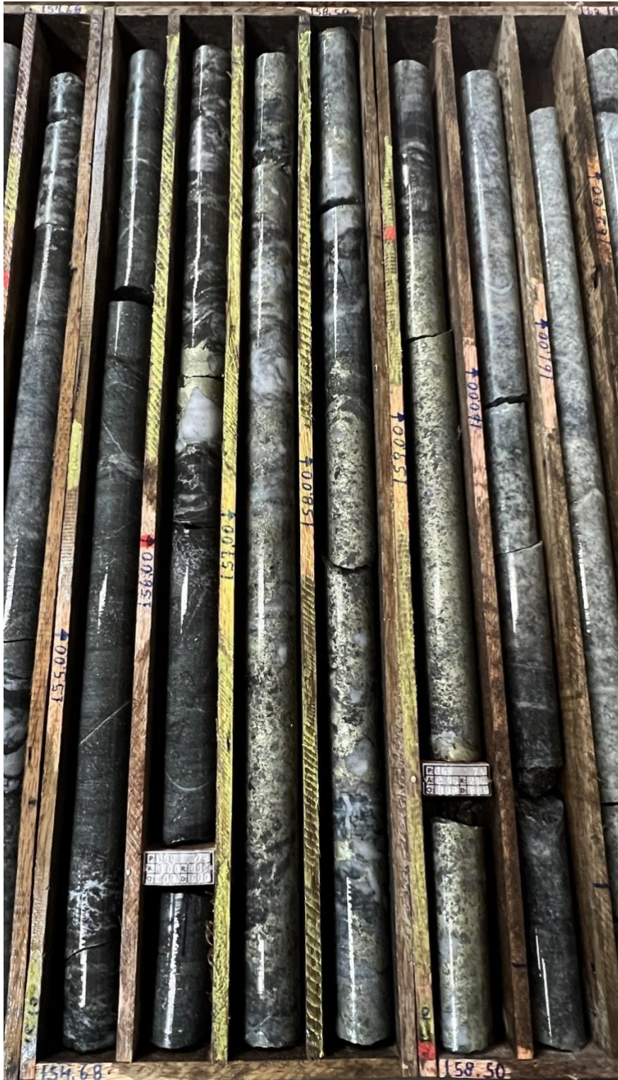
Figure 3: Semi-massive and breccia copper sulphides in DH2405T012 (154.68 – 161.25m shown).
