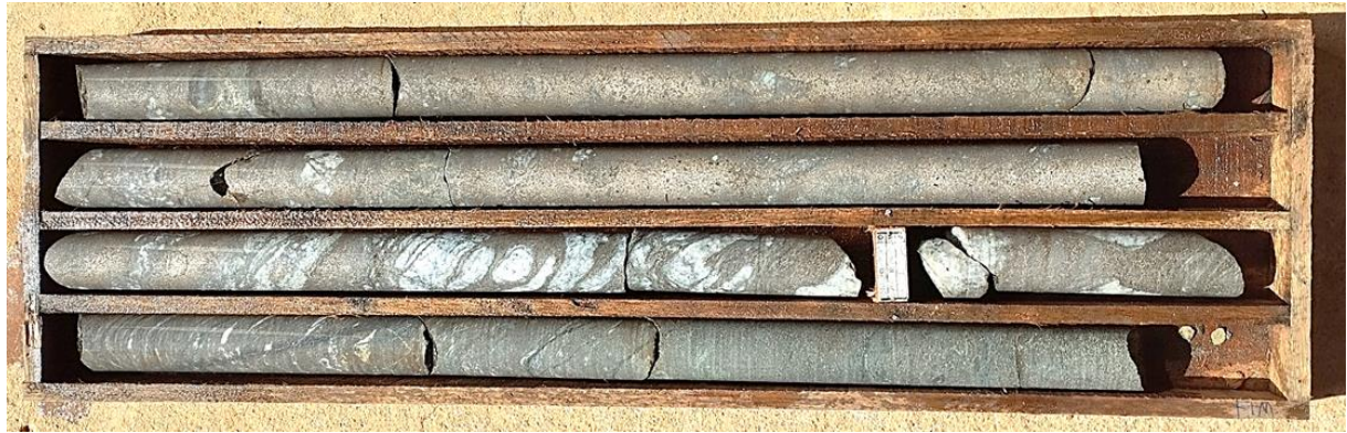
Figure 5: DDH2406T002 Massive/semi-massive/ breccia sulphide mineralization at T6 target (57.0 – 60.7m shown).
