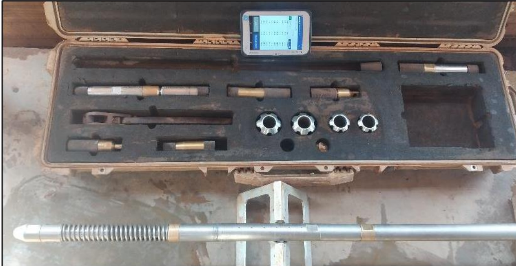
Figure 10-3: REFLEX GYRO SPRINT-IQ device used for guided run
