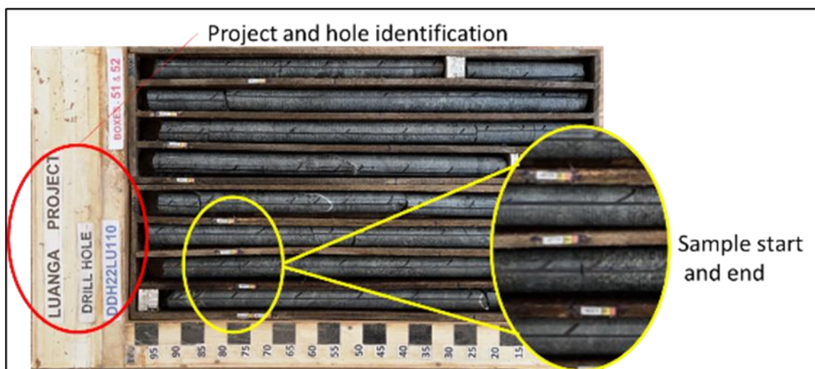
Figure 11-1: Example of photographic record of drill core box with marks and sampling ID
