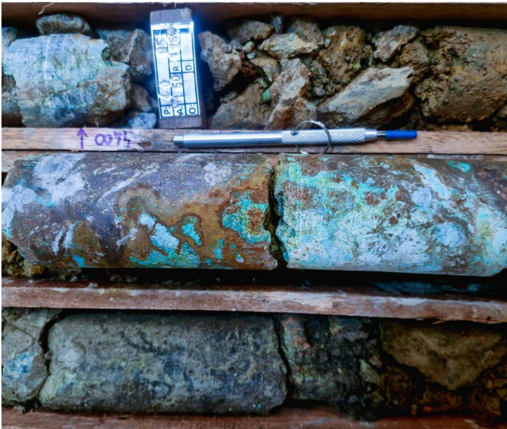
Figure 3: Mixed High-Grade Cu and PGM+Au mineralization in oxide, intercepted in DDH26LU307 (~40-42m Depth shown).
