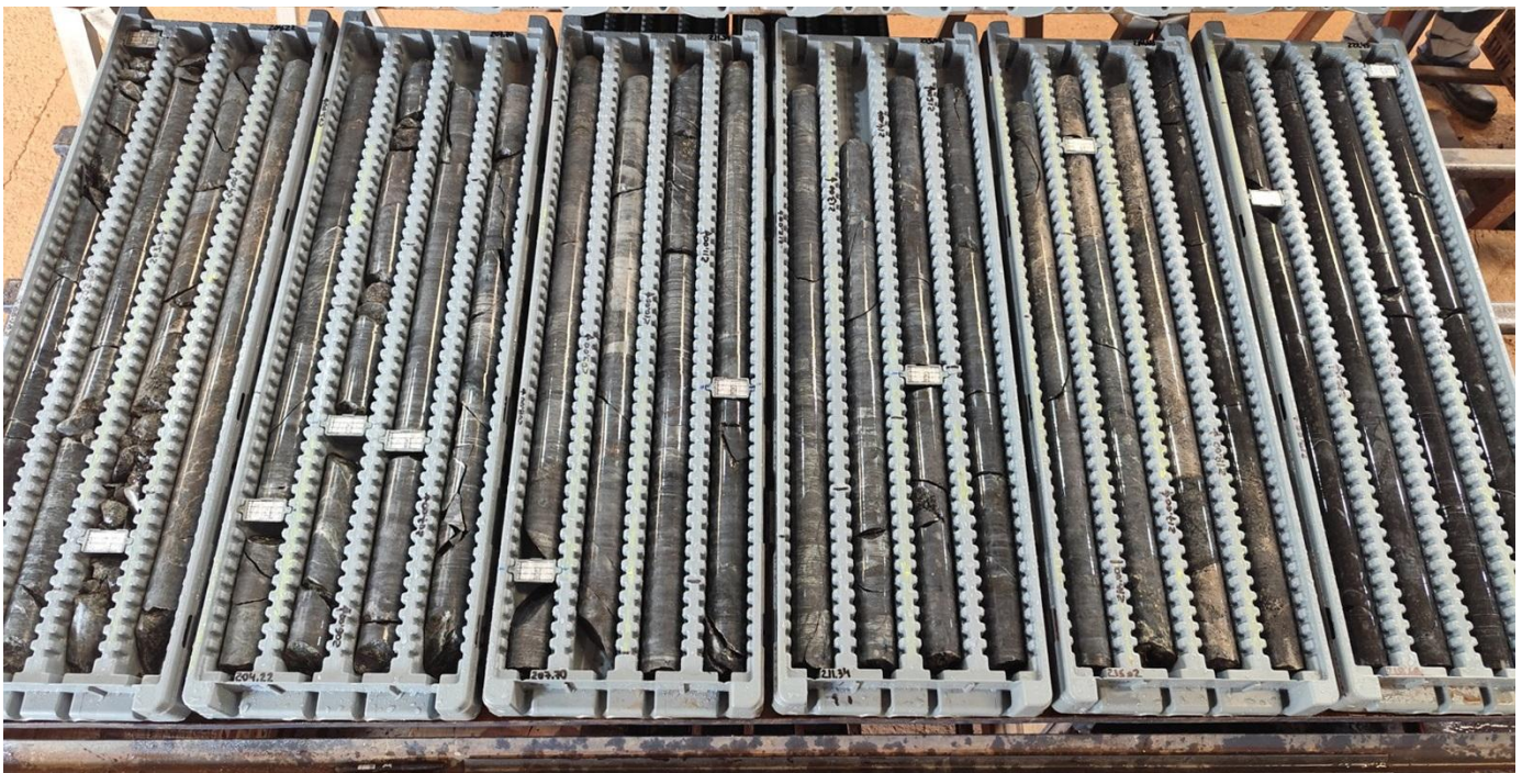
Figure 1: Sulphide-rich interval (200.53 to 222.45m) in drill hole DDH26LU330.
