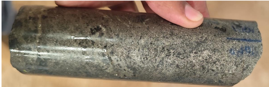
Figure 3: Harzburgite with semi-massive sulphide interval (216.60m) in drill hole DDH26LU330.
