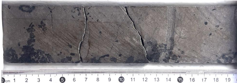
Figure 7: Massive sulphide interval (54.86 to 55.06m) in drill hole DDH25LU293.
