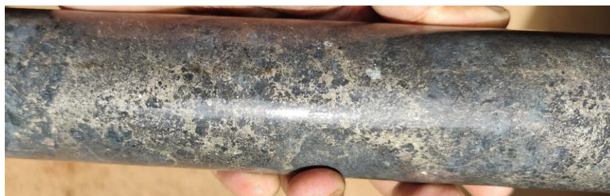
Figure 2: Harzburgite with semi-massive sulphide + chromite rich interval (203.66m) in drill hole DDH26LU330.
