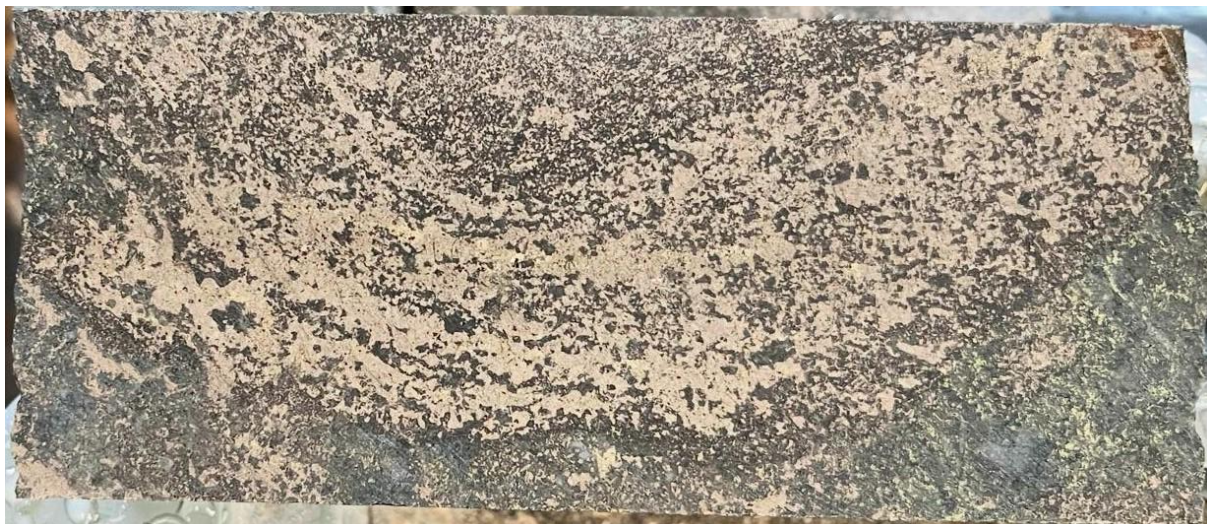
Figure 4: Banded pods of massive sulphide with chromite (208.45 – 208.55 m).
