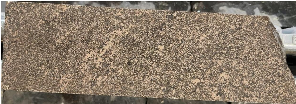
Figure 3: Massive sulphide with chromite (206.90 – 207.05 m)
