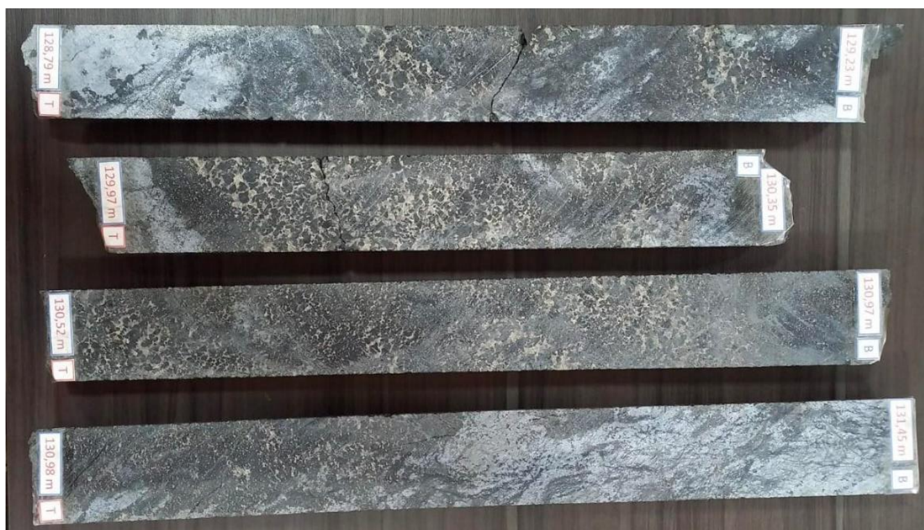
Drill Core from DDH22LU039 – Selected samples from between 128.80m and 131.50m
