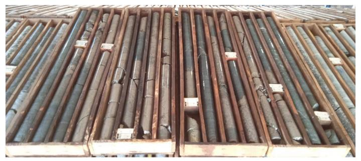
DDH22LU047: Drill core showing massive and brecciated semi massive sulphides, from 131.1m to 142.1m\*
