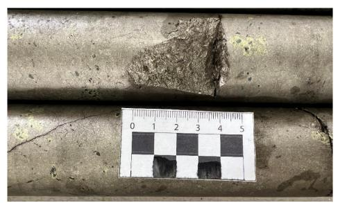
DDH22LU047: Massive sulphide mineralization interpreted as pyrrhotite + lesser pentlandite (a nickel mineral) and chalcopyrite (a copper mineral), from 136.0 to 137.6m\*
