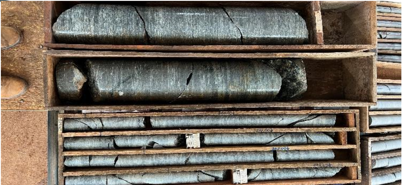
Figure 5: Geological logging of ZW size metallurgical drill core compared to regular NQ2 core.
