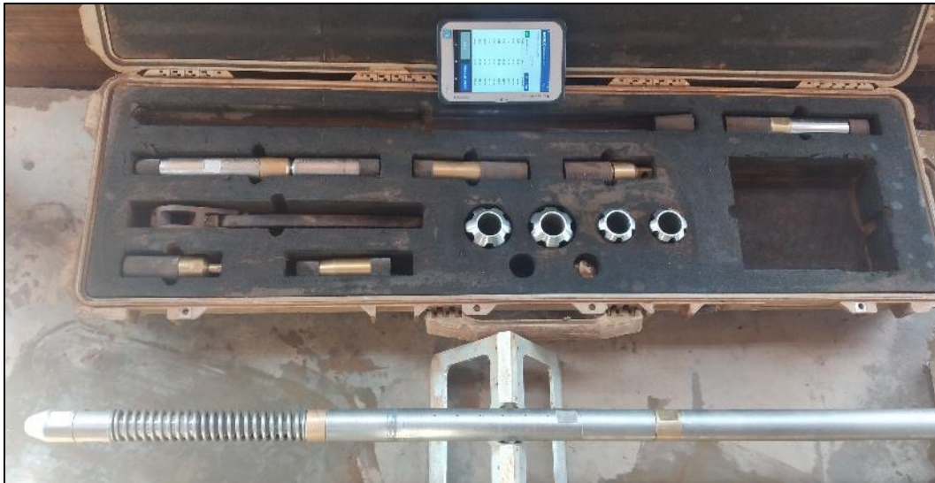
Figure 10-7: REFLEX GYRO SPRINT-IQ device used for guided run.
