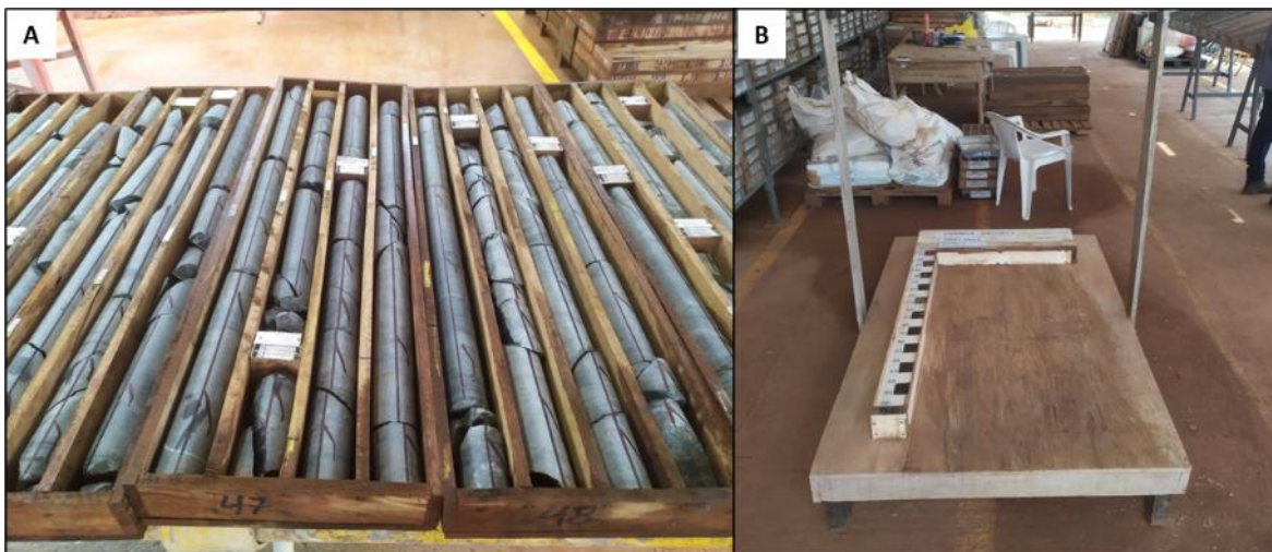
Figure 10-11: (A) Drill cores with core orientation markings and (B) Core Photography Table.
