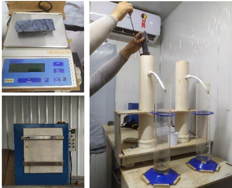
Figure 11-3: Sample density: Upper left - Scale; Bottom left – Drying oven; Right - Volume calculation.
