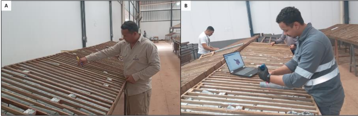
Figure 10-10: (A) Checking the core boxes and (B) taking structural measurements with IQ Logger.
